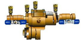
**Double Check Valve Assembly (DC)** Consists of two check valves within one body. It is essentially an RPZ minus the relief valve. The absence of the relief valve reduces the devices effectiveness. Can be used to prevent both backflow and backsiphonage, however shall only be used for to protect against pollutants only.
